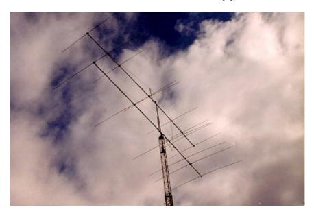
This antenna is, without doubt, the best antenna I have ever built. The side and back rejection are absolutely phenomenal and the 1.5 VSWR bandwidth through 100' of Belden 9913 extends the entire way from 20.000 MHz to 21.500 MHz! The element spacing is rather wide considering the boom length but experimentation showed that the addition of a  $7^{th}$  element did not contribute anything to the performance.
