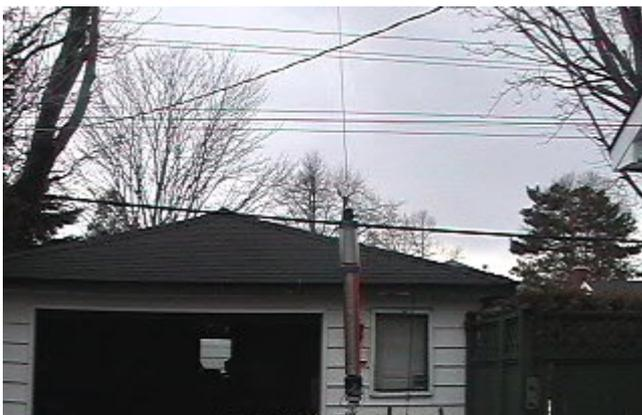
THE BOTTOM HALF OF THE TUBE IS 2.5 INCH PVC PIPE AND IS TAPED WITH COPPER FOIL USED IN STAIN GLASS PROJECTS. THE TOTAL WEIGHT IS 4 POUNDS. **I FEEL FROM MY EXPERIENCE AND EXTREME WX CONDITIONS THE PVC PIPE IS STRONG ENOUGH FOR MOBILE OPERATION.**
