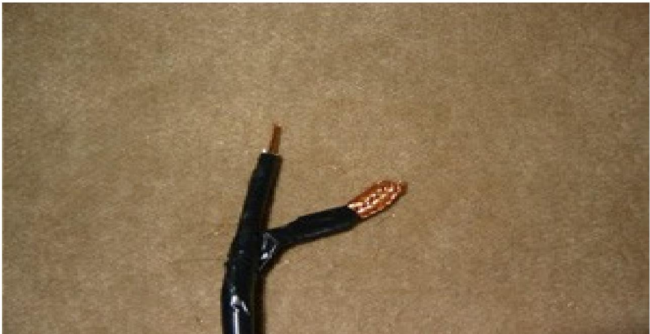
This is important, leave a half inch or so of center conductor without tape so you can cut off the white dielectric and expose the copper inside for attachment to the loop. I would recommend using a wire cutter for this, and gently pull off the white covering on the center conductor. You now should have a stub with a nice Y with both braid exposed and the an exposed center conductor. This is the part of the coaxial stub that will eventually be attached to the loop.
