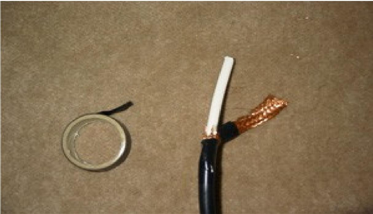
.Once you have this re-enforcing tape on the braid, tape up the rest of the braid as shown leaving a half inch exposed This will give you a nice strong Y at the end of your coax for attachment to the loop. Also tape of the outside white foam dielectric of your cable too. I beleive each layer of electrical tape has a 1 KV tolerance, so let's beef up the coax a bit anyway. I have seen the white foam dielectric melt at high wattage and burn and vaporize -- so it can't hurt!
