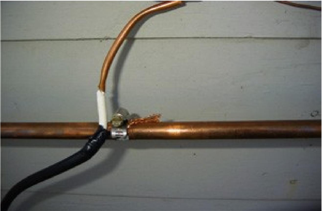
Take your copper wire or thin copper pipe and get ready. Strip off the center conductor dielectric for about 1/2 an inch. Take your thick copper wire or thin copper pipe -- it should be around 10 inches long -- and wrap it around your center conductor wire, or place your thick copper pipe over the center conductor of the coax and crimp it on with a tool. You can also solder the connection, but use low heat so you don't burn the coax, or the dielectric. Now we'll complete the loop.
