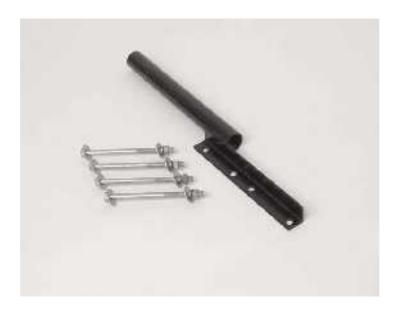
The bracket shown was fabricated to provide a proper mounting point for the Yaesu G-800SA rotator.
