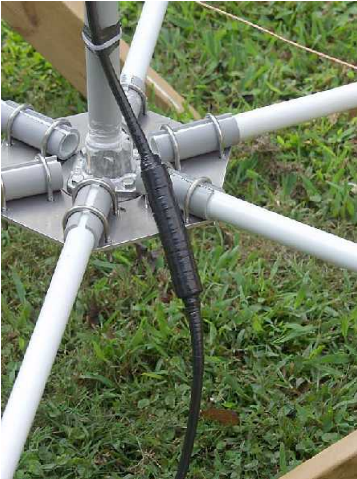
This is the HexBeam base. Everything attaches to that big hexagonal aluminum plate. The black blob on the RG-213 feedline is an RF choke, made from six Amidon FB-77-1024 Ferrite cores, wrapped up and weatherproofed.
