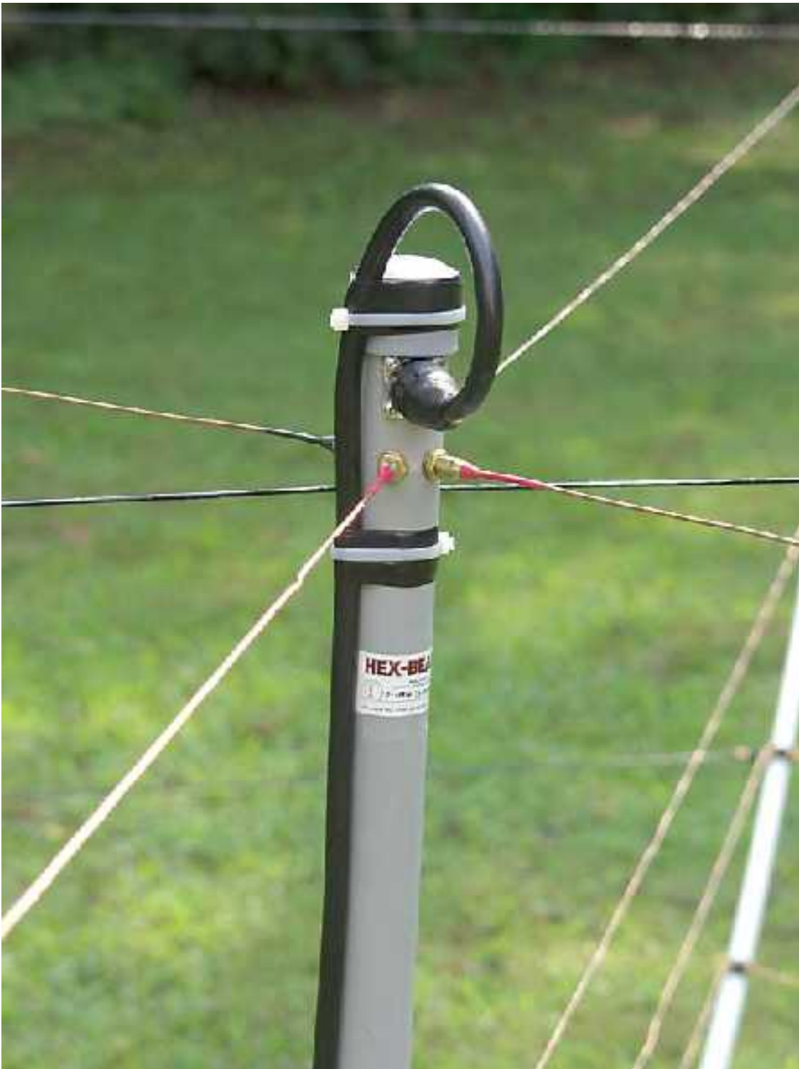
This is the feedpoint of the HX-B5i HexBeam. the red wires shown here are the 20 M driven element, and the black wires are the 20 M reflector.
