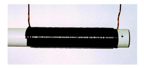
Figure 4—Wrap the coil in electrical tape.
